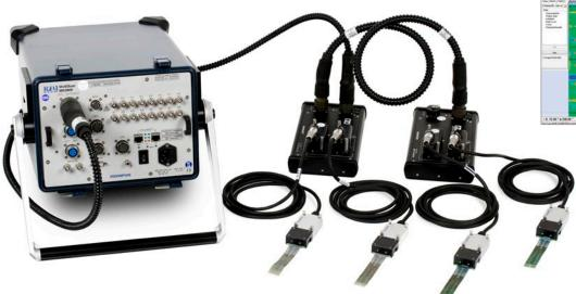
Example of MS5800 system with 4x 32-channel ECA probes connected through 2 ECA multiplexers.
